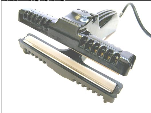
**KF-150PS** is a poly heat sealer. It makes a perfect strong 6" long and 1/18" wide seal on poly bags and other thermoplastic materials. The upper jaw holds the metal sealing bar with a 275°F sealing temperature and is covered with a Teflon cloth. The bottom jaw holds the resilient silicon rubber. This sealer seals polyethylene or polypropylene up to 6 mil thick.
