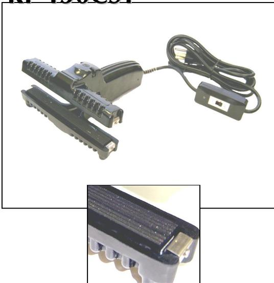
**KF-150CST** is a direct heat sealer equipped with 2 heated 9/16" (15mm) wide and 6" long Teflon coated, serrated (horizontal line seal imprint) jaws. It is ideal for sealing cellophane, coated aluminum foil, Kraft paper, and other thick materials. The temperature switch has 2 temperature settings, 350 & 450 ° F. It can be used as a heat sealer.
